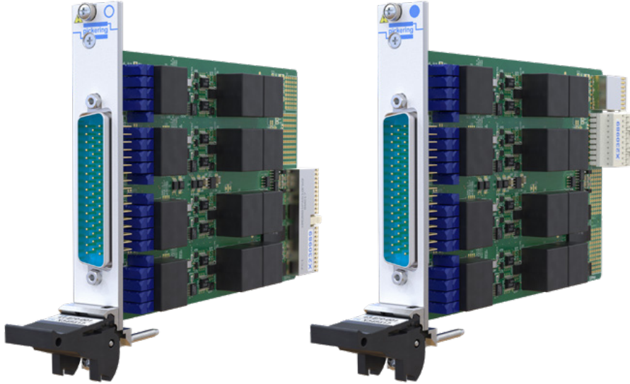
Figure 8 - Pickering Interfaces' LVDT/RVDT/resolver simulator modules 41-670 (on the left) for PXI and 43-670 for PXIe (on the right).
