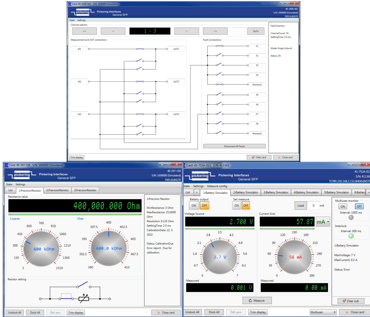
Example of soft front panels for simple operation of individual modules
